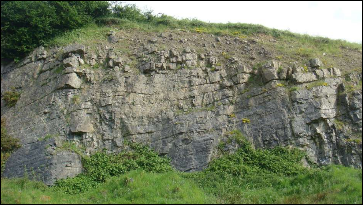
Plate 7-5: Typical profile of shallow depth to bedrock, with thin weathered zone at the top of rock (access road into quarry)
