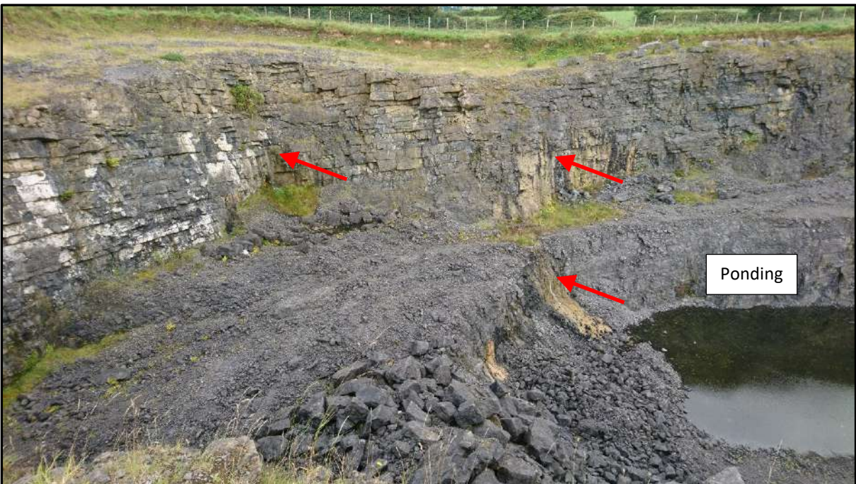
Plate 7-16: Groundwater inflows from epikarst at northwest corner of quarry (photographed from above Plate 7-15 location)
