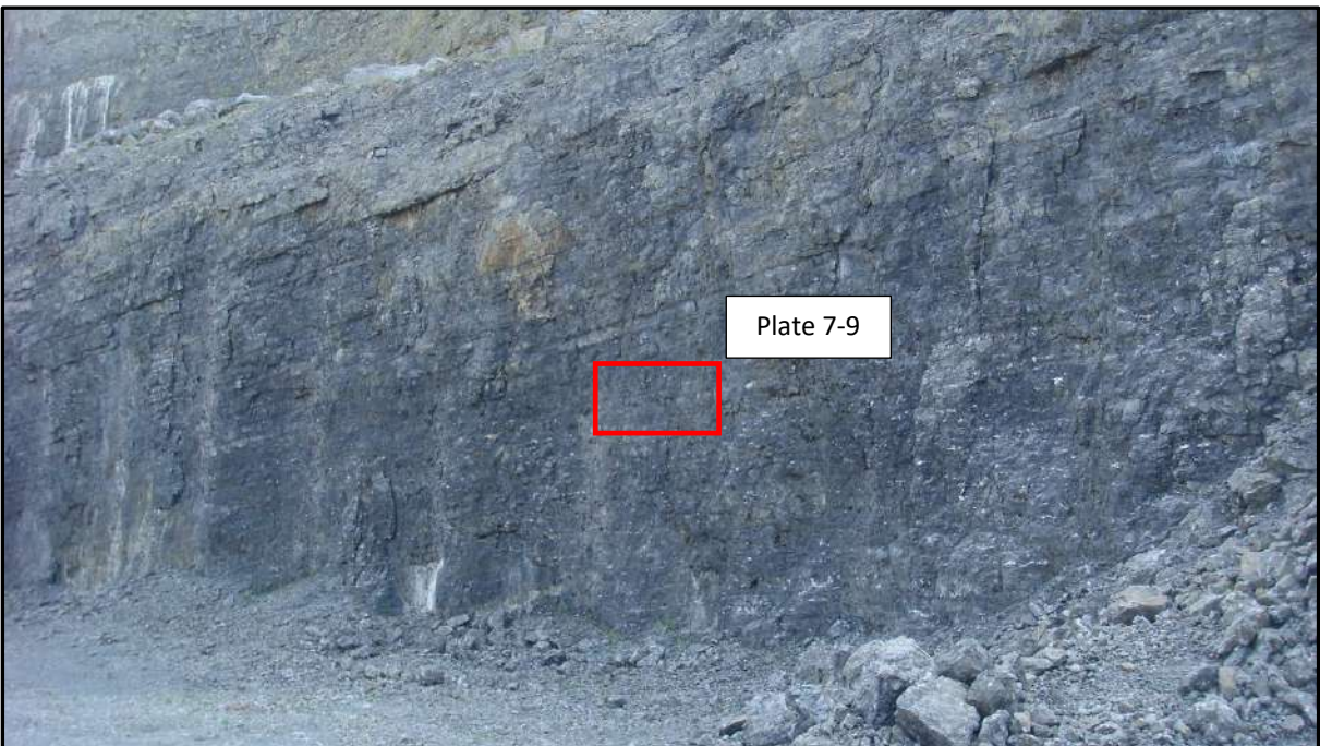
Plate 7-8: Massive limestone beds with weathered 'vuggy' cavities delineating bedding
